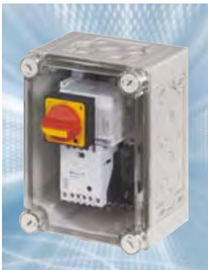
Figure 4: Small switchgear assembly with the PKZ 2 motor-protective circuit-breaker providing all switching and protective functions on a simple machine, including main switch and emergency-stop function.
