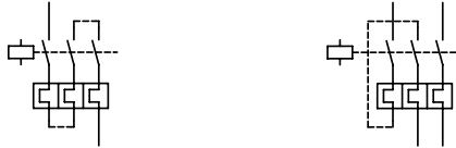
Figure 6: Wiring of the motor-protective relay for the protection of AC or DC motors (bimetallic release switched in series)
