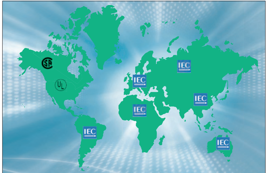
Photo 1: Globally, the great majority of electrical components and assemblies conform to IEC standards. In the US and Canada, the UL and CSA standards help to insure compliance with the NEC and CEC, which are the relevant installation standards in that region.
