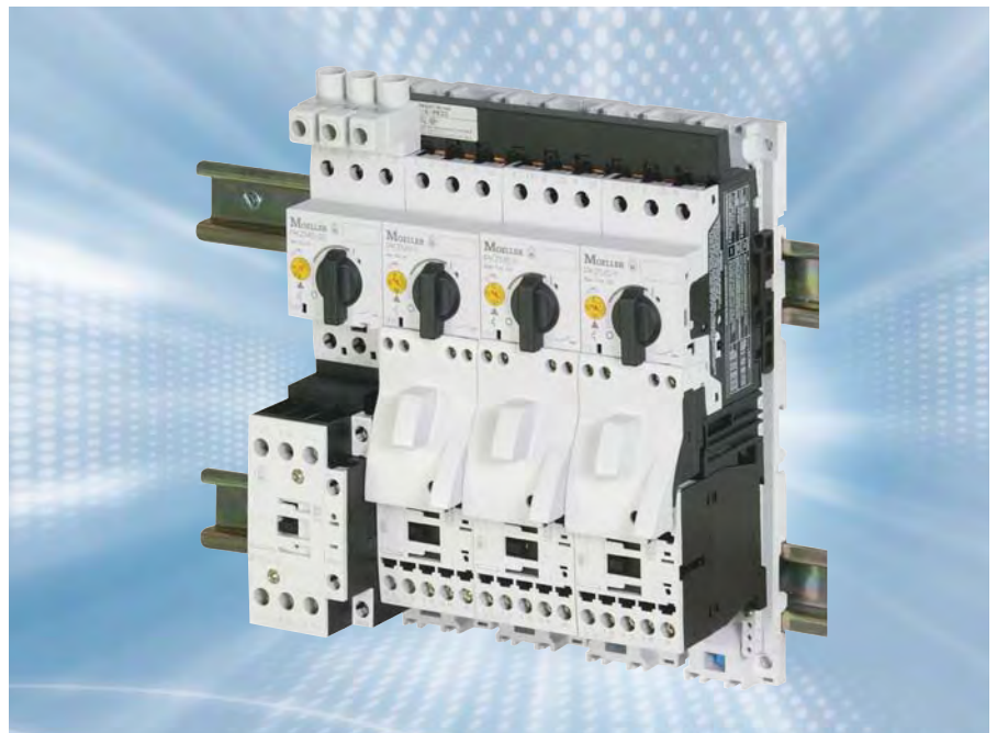
Figure 4: Examples for "Type F Combination Motor Starters" which result from tested combinations of self-protected manual "Type E" devices and magnetic contactors.
