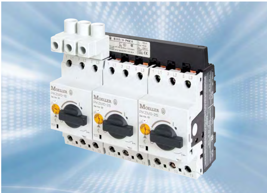
Figure 3: Motor-protective starters/circuit-breakers PKZM0 with power feed side three-phase bus commencing links. The common power feed terminal BK25...-E constructionally fulfills the larger supply side clearances needed for "UL 508 Combination Motor Starters of Construction Type E".
