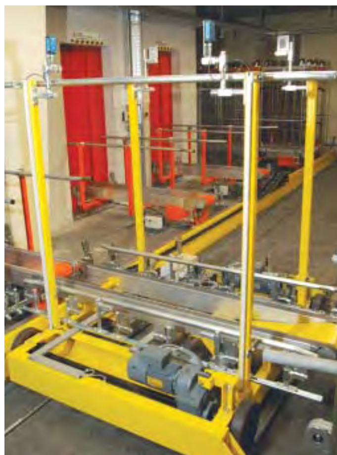
The decision as to which type is to be sent on which route is made on the transverse shuttle car. The entrances to the two lifts can be seen in the background.
