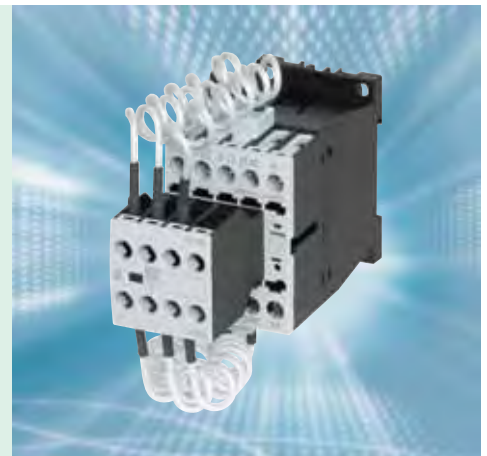
Bild 10: Special Type DIL K capacitor switching contactors can be used to switch banks of capacitors for power factor compensation purposes. The charging resistors reduce the extremely high inrush current peaks. Regular DILM contactors can be used for individual compensation or when capacitor banks are equipped with inductive choking means.
