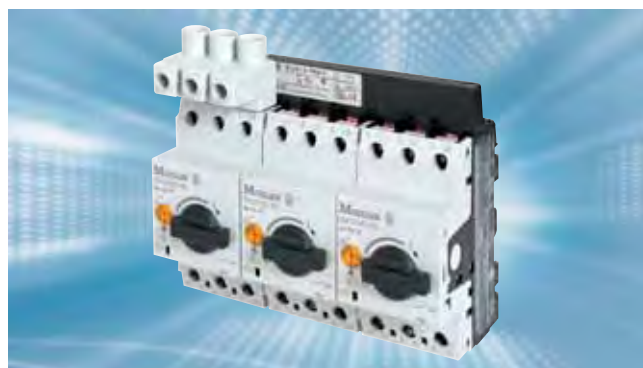
Photo 4: A PKZM0 motor protective starter grouping is linked on its supply side via a 3 phase bus connector bus. The motor protectors are fed using a common incoming terminal block BK25...-E, which features larger, distribution size electrical clearances to fulfill the requirements of a „Type E construction“.
