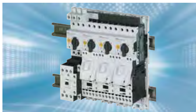
Photo 5: Examples of UL 508 Type F Combination Starters, which consist of UL 508 manual self-protected Type E Combination controllers combined with standard magnetic contactors.
