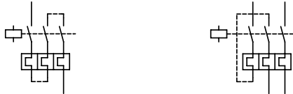
Figure 5: Wiring of the motor-protective circuit-breaker for the protection of AC or DC motors (bimetallic release switched in series)
