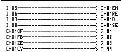
Figure 104: MFD-Titan circuit diagram with high-speed counter
