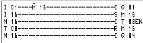
Figure 194: Automatic reset of error signal
