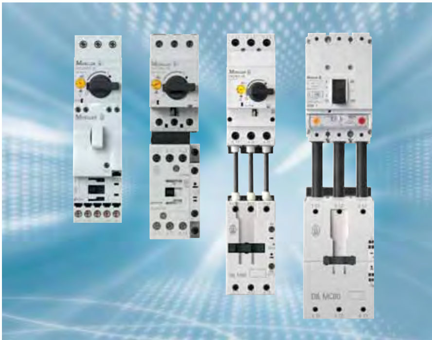
Photo 2: Universally applicable World Market rated contactors for the xStart Product Range. The motor starters rated up to 150A are ideally suited for normal industrial motor switching but the contactors themselves can be applied just as well in North America for „Special Purpose applications“.
