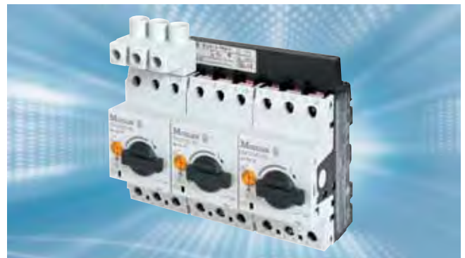
Photo 4: A PKZM0 motor protective starter grouping is linked on its supply side via a 3 phase bus connector bus. The motor protectors are fed using a common incoming terminal block BK25...-E, which features larger, distribution size electrical clearances to fulfill the requirements of a „Type E construction“.
