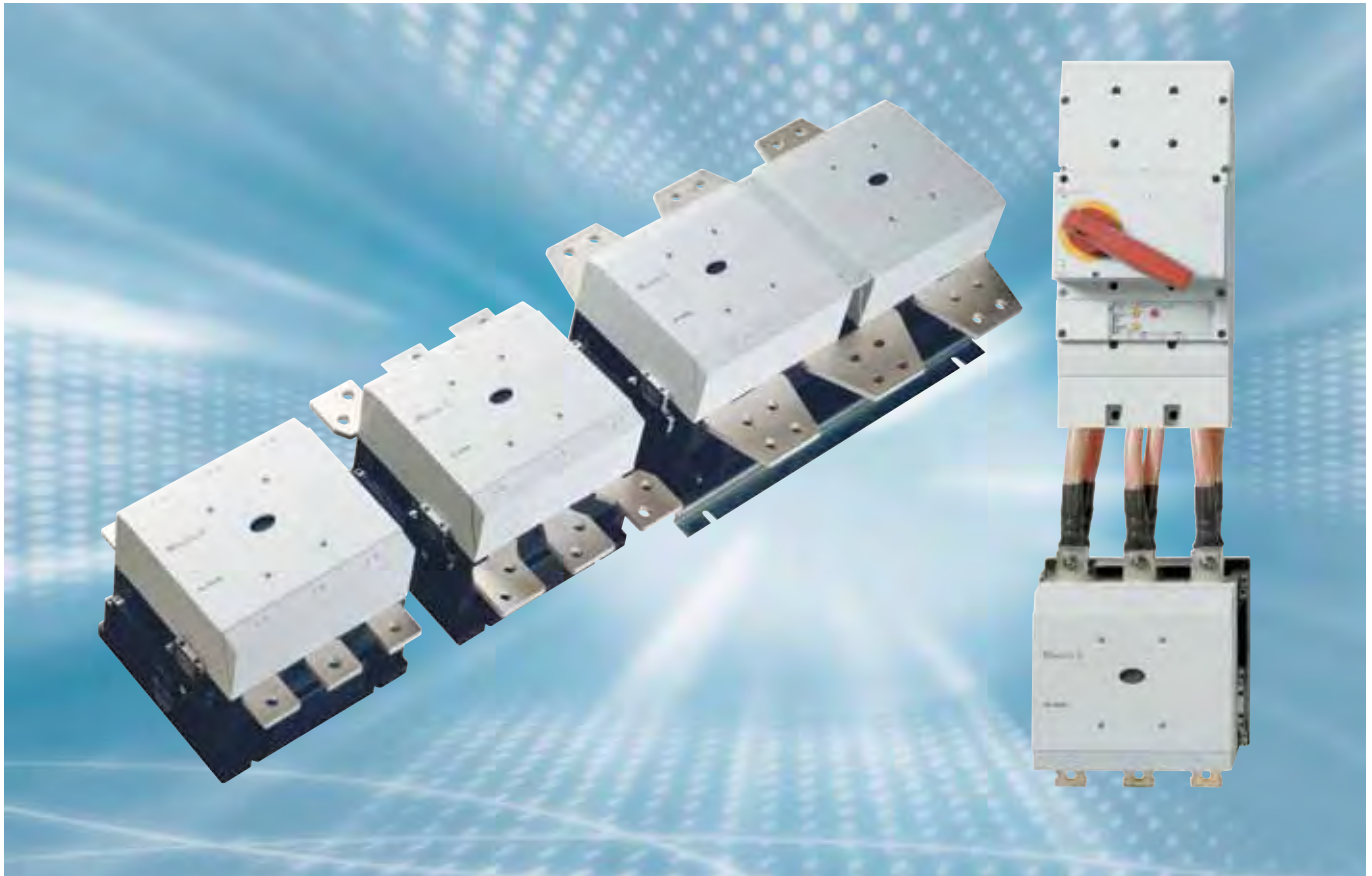
Photo 3: For larger size contactors Moeller has now for years been employing vacuum technology [12] rather than using air as a medium for switching contacts, thus enabling higher component life and reducing overall dimensions. Most of them are applied in motor starter combinations.
