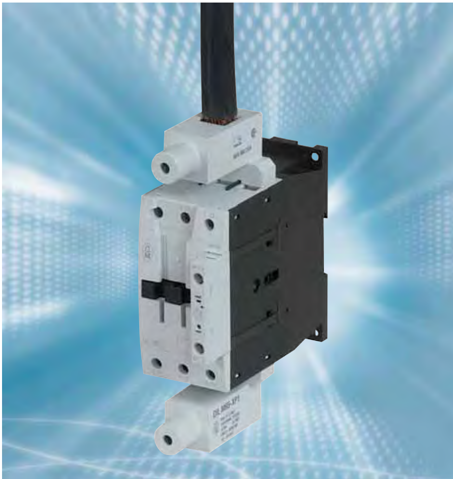
Photo 9: The paralleling bridge allows the AC-1 „General Purpose“ 3 phase current rating of the contactor to be increased by a factor 2.5 times its value. This accessory is especially useful when switching single phase resistive loads (such as heaters). It permits the use of smaller, and more economical, contactors to handle the load.
