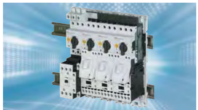
Photo 5: Examples of UL 508 Type F Combination Starters, which consist of UL 508 manual self-protected Type E Combination controllers combined with standard magnetic contactors.
